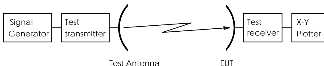
Figure 9: Test arrangement - antenna transmit radiation pattern measurement
