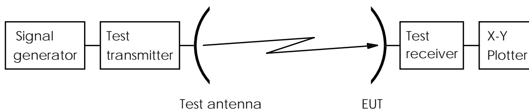
Figure 10: Test arrangement - transmit polarization discrimination
