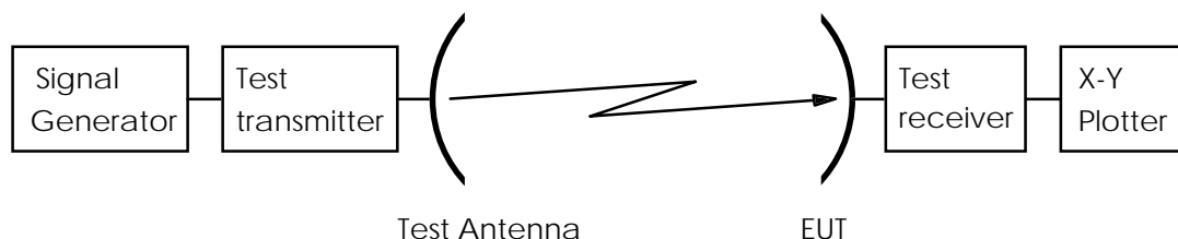
Figure 9: Test arrangement - antenna transmit radiation pattern measurement
