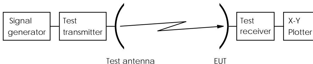
Figure 10: Test arrangement - transmit polarization discrimination
