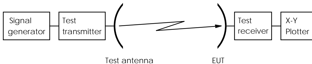
Figure 7: Test arrangement - transmit polarization discrimination
