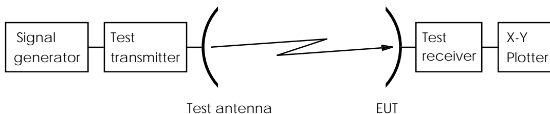
Figure 10: Test arrangement - transmit polarization discrimination
