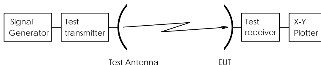
Figure 9: Test arrangement - antenna transmit radiation pattern measurement
