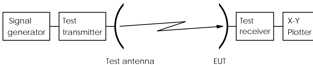
Figure 10: Test arrangement - transmit polarization discrimination
