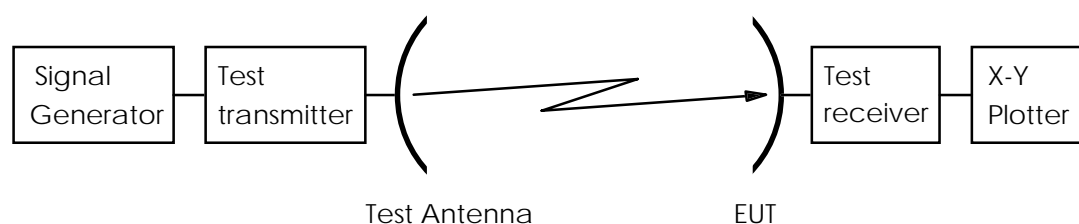
Figure 9: Test arrangement - antenna transmit radiation pattern measurement
