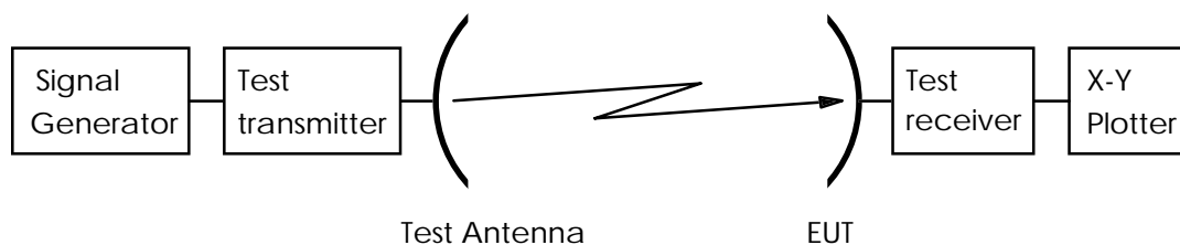
Figure 9: Test arrangement - antenna transmit radiation pattern measurement
