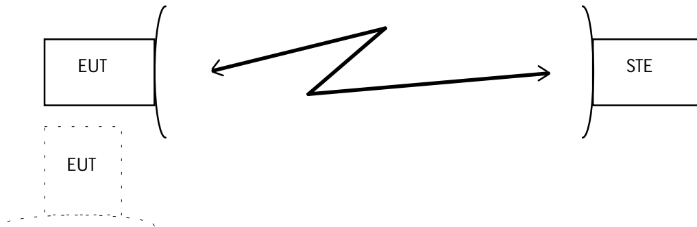
Figure 12: Test arrangement - static rms pointing accuracy
