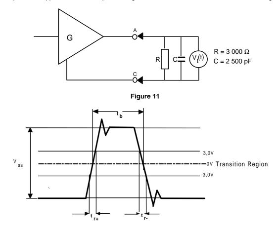
Vss=Voltage difference between steady-state signal conditions; tb=nominal duration of a bit.
