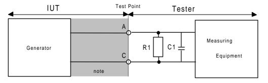
NOTE: The shaded area denotes an interconnection means e.g. interface cable and connector.
