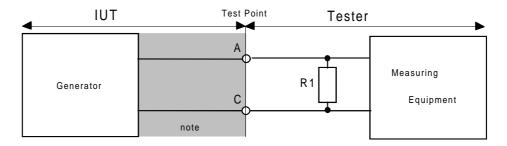
NOTE: The shaded area denotes an interconnection means e.g. interface cable and connector.
