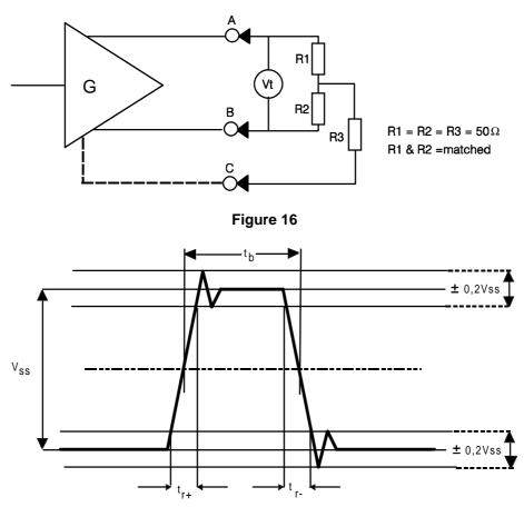
Vss=Voltage difference between steady-state signal conditions; tb=nominal duration of a bit, tr  $\leq$  0,1 tb.
