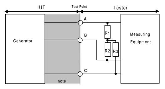
NOTE: The shaded area denotes an interconnection means e.g. interface cable and connector.
