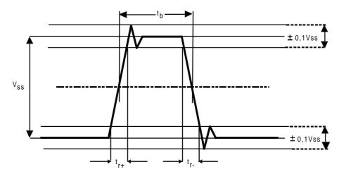
Vss=Voltage difference between steady-state signal conditions; tb=nominal duration of a bit. For tb  $\ge$  50µs, tr  $\le$  0,3 tb.
