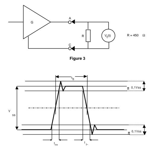
Vss=Voltage difference between steady-state signal conditions; tb=nominal duration of a bit. For tb  $\ge 50\mu$ s, tr  $\le 0.3$  tb.
