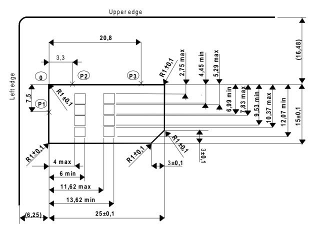
NOTE: The Plug-in SIM may be "obtained" by cutting away excessive plastic of an ID-1 SIM. The values in parenthesis in figure A.1 show the positional relationship between the Plug-in and the ID-1 SIM and are for information only.
