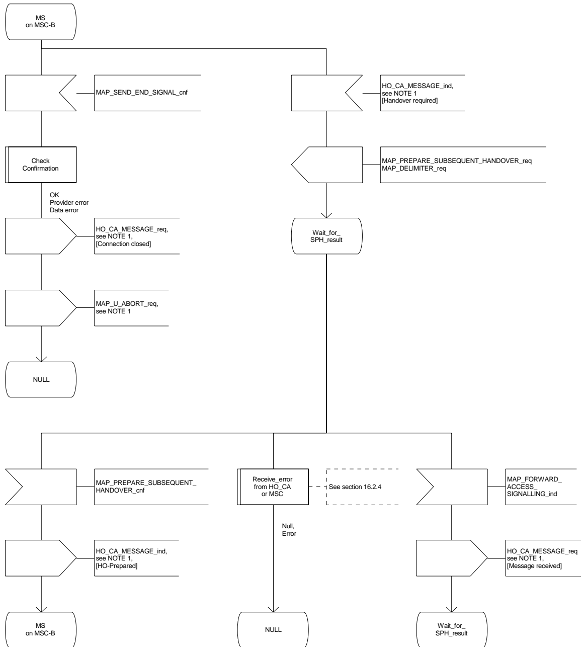
Figure 16.2.3/1 (sheet 11 of 11): Process MSC_B_HO
