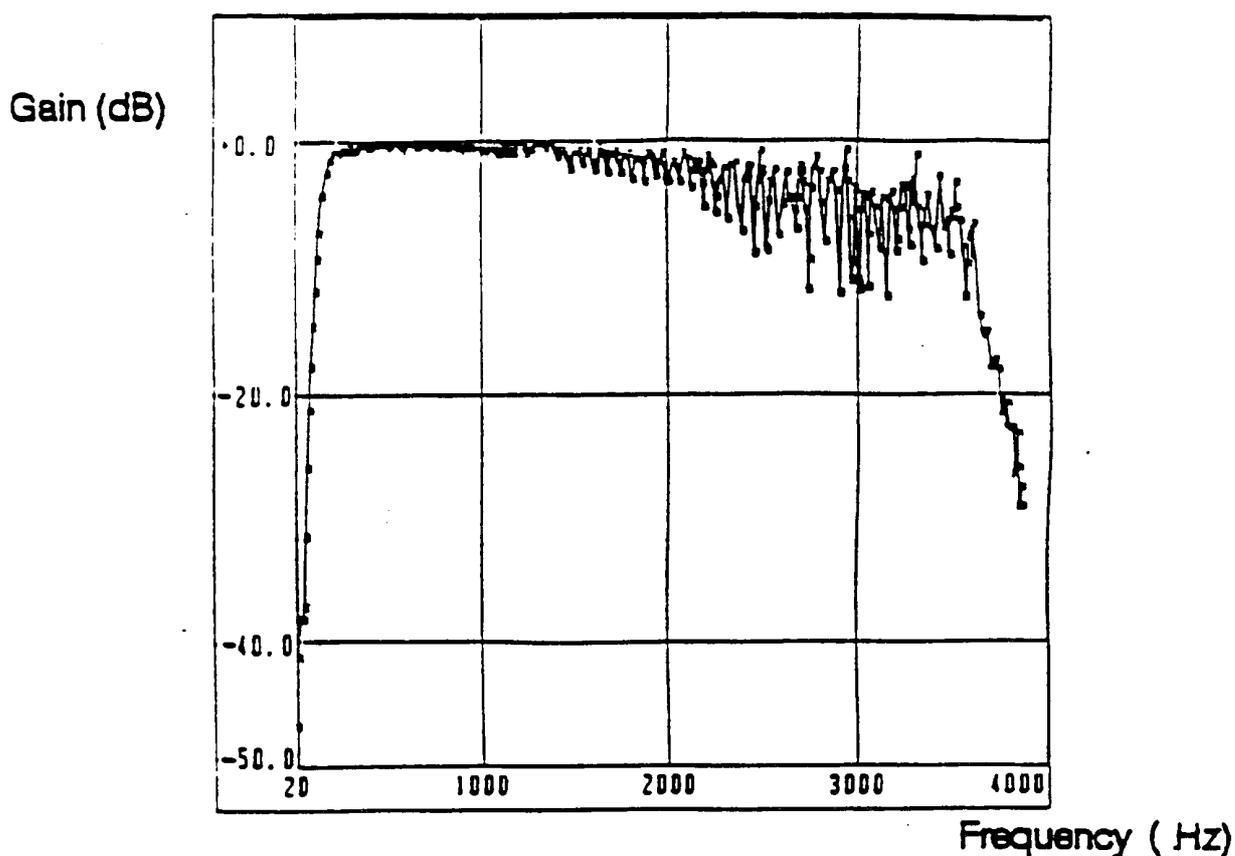
Figure A.1.5: Frequency response for RPE-LTP codec
