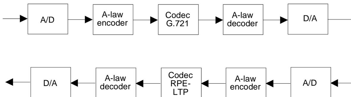
Figure A 1.4: Mixed transcodings - scheme 2
