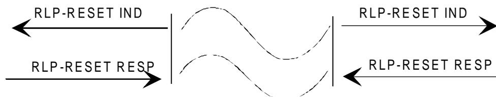
l) simultaneous user and provider invoked reset
