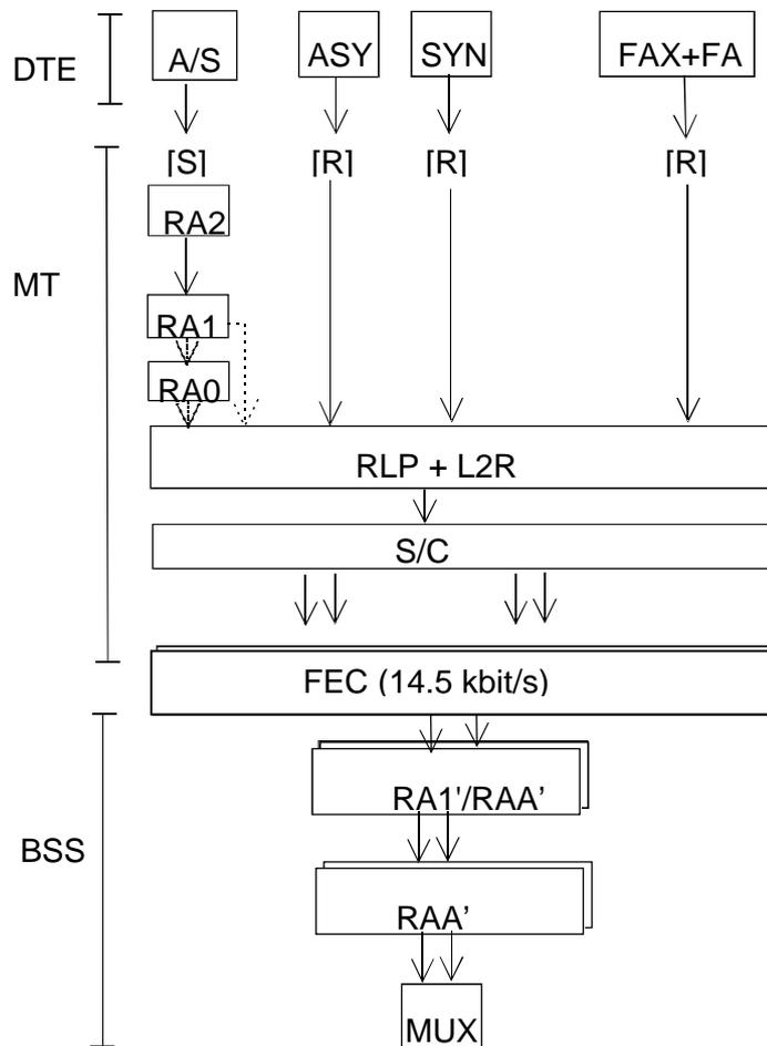
**Annex B (informative): An example of mapping Network Independent Clocking information for TCH/F14.4 when the S-interface is deployed:**
