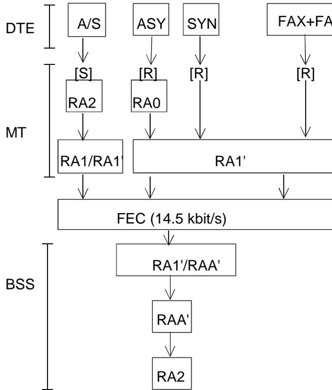
For the non-transparent services, the following stacks of rate adaptation and functions are possible:
