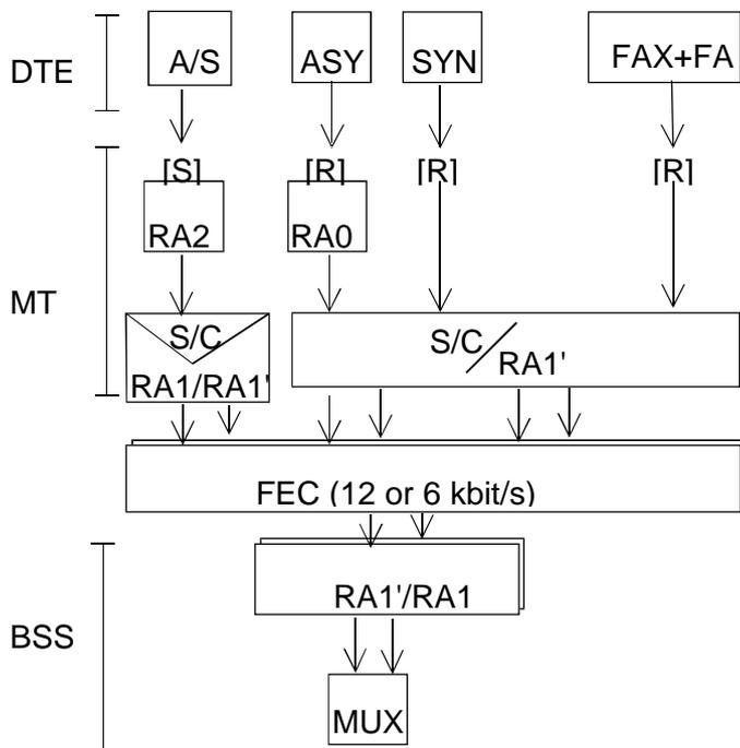
For the non-transparent services, the following stacks of rate adaptation and functions are possible:
