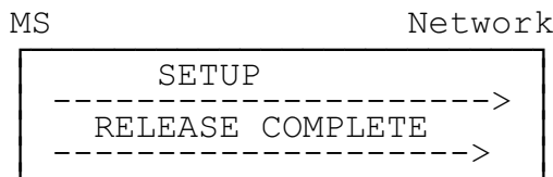
Figure 5.7b/GSM 04.08 Recall acceptance or rejection by user
