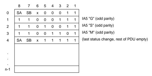
Figure 2a Single-link RLP and multi-link RLP with status octet transfer in PDU.
