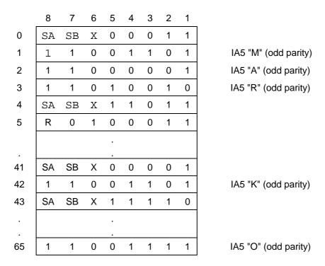
Figure 2c A 66-octet RLP L2RCOP PDU with status octets separated by more than 23 octets
