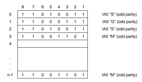
Figure 2b Multi-link RLP L2RCOP PDU with no status octet transfer
