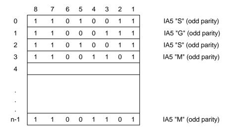
Figure 2b Multi slot RLP L2RCOP PDU with no status octet transfer
