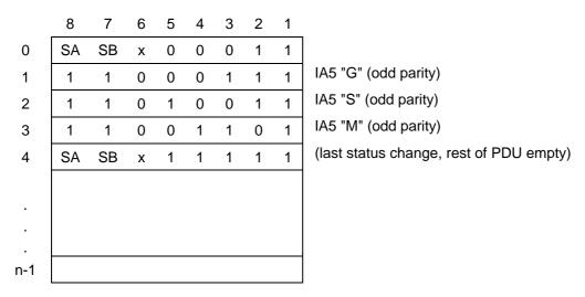
Figure 2a Single slot RLP (n=25) and multi slot RLP (n=24) with status octet transfer in PDU.
