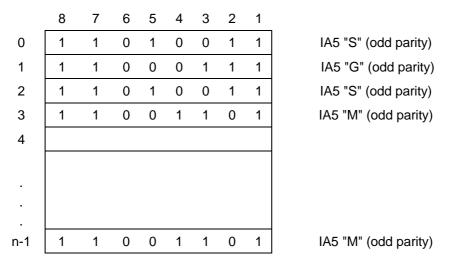
Figure 2b Multi slot RLP L2RCOP PDU with no status octet transfer
