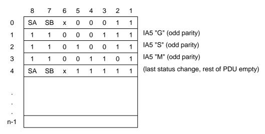
Figure 2a Single slot RLP (n=25) and multi slot RLP (n=23) with status octet transfer in PDU.
