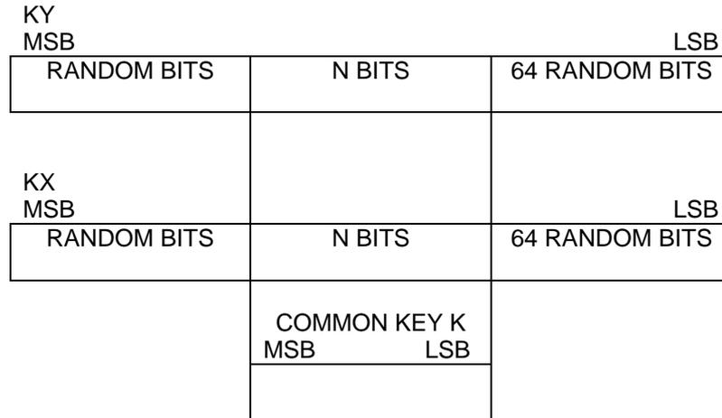
N bit blocks from KX and KY are modulo 2 added to form common Key K
