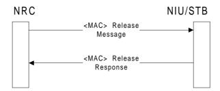
Figure 31: Connection release signalling
