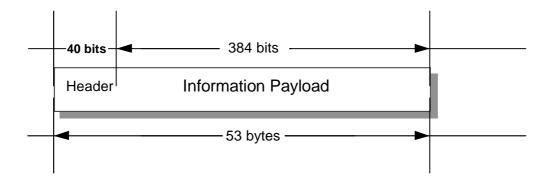
Figure 20: ATM cell format
