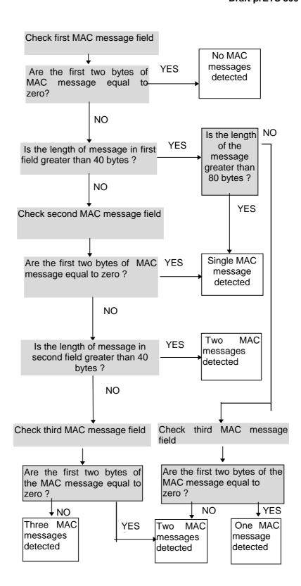
Figure 25: Algorithm when MAC message are sent IB Downstream
