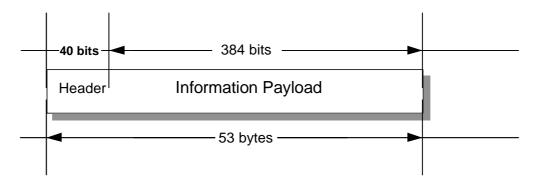
Figure 16: ATM cell format
