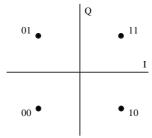
Figure 8: Mapping for the QPSK constellation (downstream OOB)
