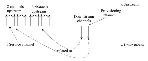
Figure 24: Example of frequency allocation
