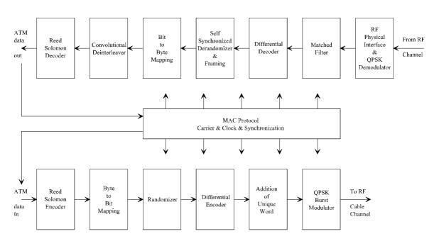
Figure 4: Conceptual block diagram for the NIU OOB Transceiver
