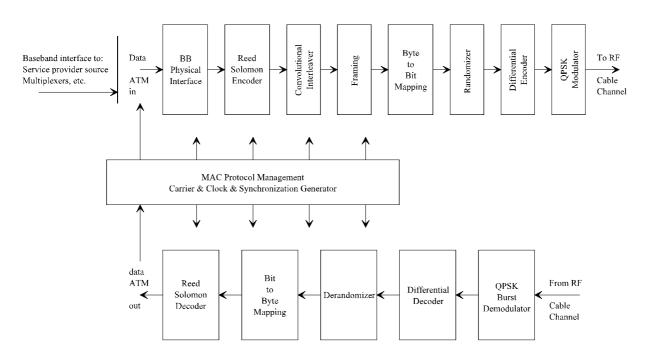
Figure 5: Conceptual block diagram for the OOB Head-end Transceiver
