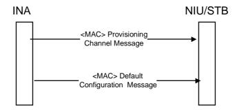
Figure 26: Initialization and Provisioning signalling
