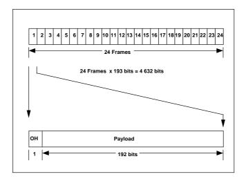
Figure 15: SL-ESF frame structure
