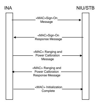
Figure 27: Ranging and Calibration Signalling
