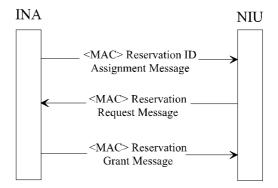
Figure 32: Reservation access signalling
