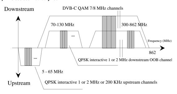
Figure 3: DVB preferred frequency ranges for CATV interactive systems
