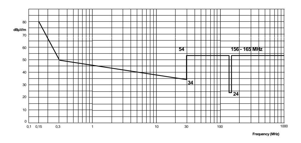
Figure 1: Maximum level of field strength of unwanted emissions at 3 m distance
