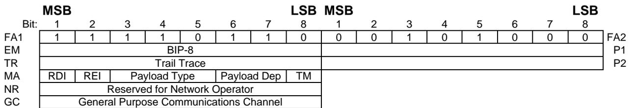
**Figure C.2: Path overhead at 139 264 kbit/s**
