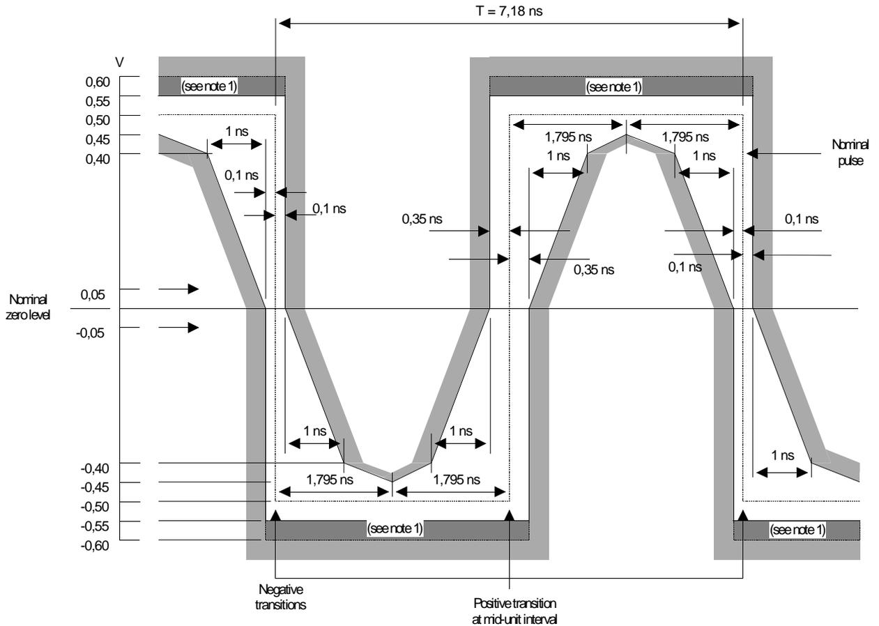
NOTE 1: The maximum "steady state" amplitude shall not exceed the 0,55 V limit. Overshoots and other transients are permitted to fall into the dotted area, bounded by the amplitude levels 0,55 V and 0,60 V, provided they do not exceed the steady state level by more than 0,05 V.
