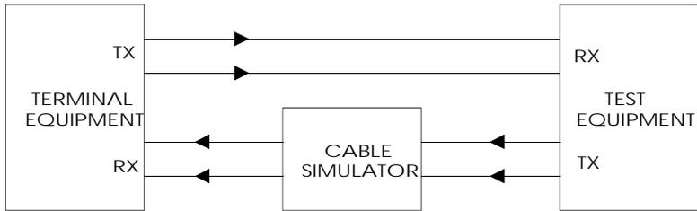
**Figure A.4: Input coding and loss tolerance**
