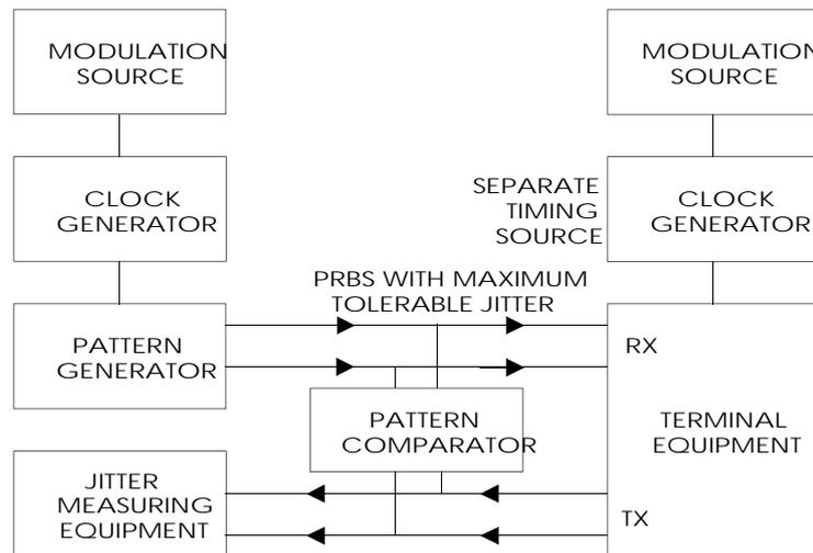
NOTE: The modulation source may be included in the clock generator and/or the pattern generator, or it may be provided separately.
