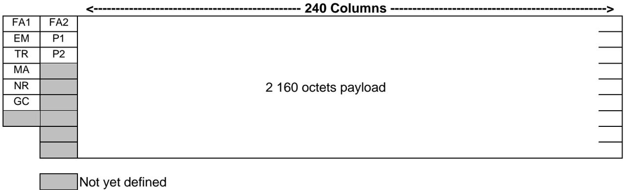
**Figure C.1: Frame structure at 139 264 kbit/s**
