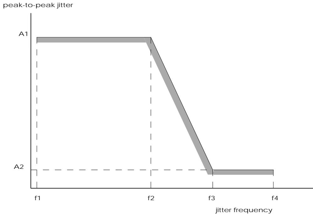
Figure 4: Input jitter tolerance
