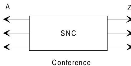
Figure D.4: Broadcast and conference sub-network connections
