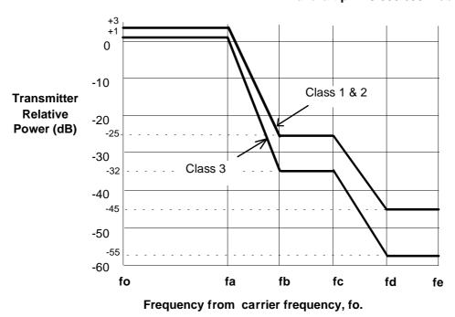
**Channel Spacing** fb fa fc fd fe 500 kHz 210 kHz 325 kHz 450 kHz 800 kHz 1 250 kHz 1 MHz 420 kHz 650 kHz 900 kHz 1 600 kHz 2 500 kHz 1,75 MHz 750 kHz 1 150 kHz 1 600 kHz 2 800 kHz 4 375 kHz 2 MHz 840 kHz 1 300 kHz 1 800 kHz 3 200 kHz 5 000 kHz 1 500 kHz 3 500 kHz 6 000 kHz 8 750 kHz 3,5 MHz 2 400 kHz 7 MHz 3 000 kHz 4 800 kHz 7 000 kHz 12 000 kHz 17 500 kHz 14 MHz 6 000 kHz 9 600 kHz 14 000 kHz 24 000 kHz 35 000 kHz
