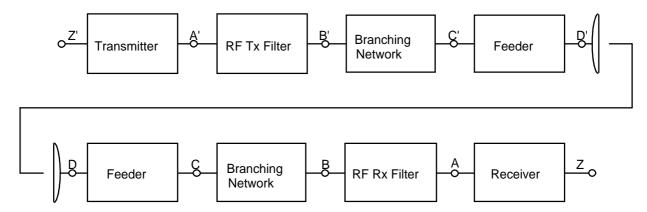
NOTE 1: For the purpose of defining the measurement points, the branching network does not include a hybrid.
