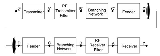
NOTE 1: For the purpose of defining the measurement points, the branching network does not include a hybrid.
