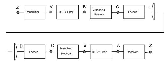
NOTE 1: For the purpose of defining the measurement points, the branching network does not include a hybrid.
