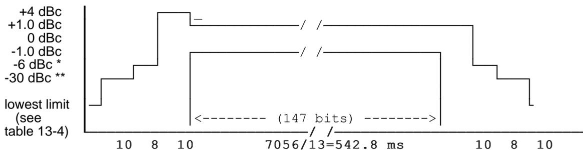
Figure 13-1: Power / time template for normal bursts
