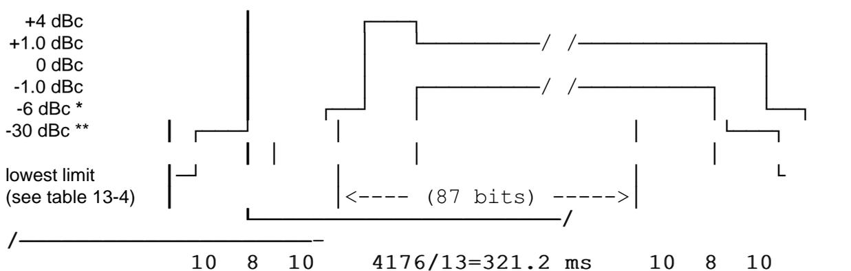
Figure 13-2 : Power / time template for access burst
