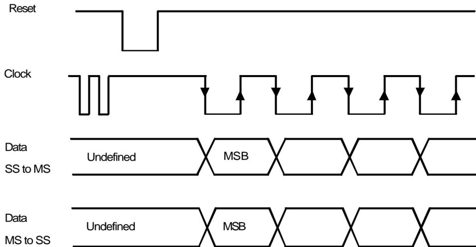
Figure 36-2 / GSM 11.10 : DAI Timing
