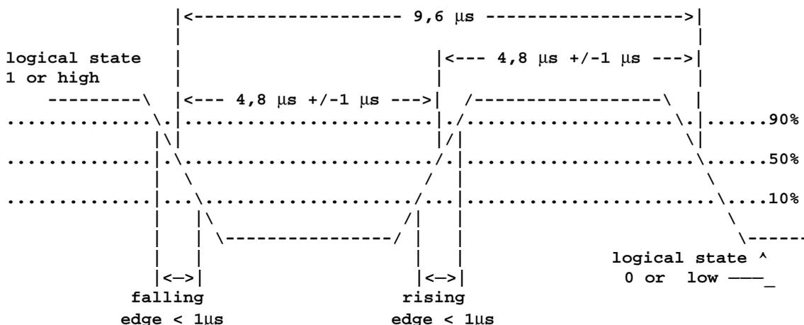
Data shall be stable during the period between 3 microseconds before and 1 microsecond after the rising edge of the clock (50% level).
