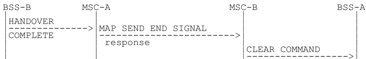
Figure 14: Signalling for Subsequent Inter-MSC Handover back to MSC-A completion (Successful completion of the procedure)
