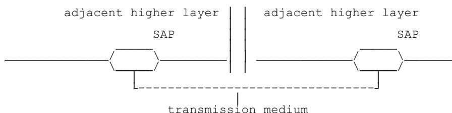
Figure 3.1: Service Access Point principle
