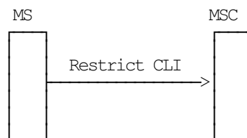
Figure 2.2: MS invoking CLIR, when CLIR is provisioned in temporary mode with default value "presentation allowed"
