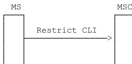
Figure 2.2: MS invoking CLIR, when CLIR is provisioned in temporary mode with default value "presentation allowed"
