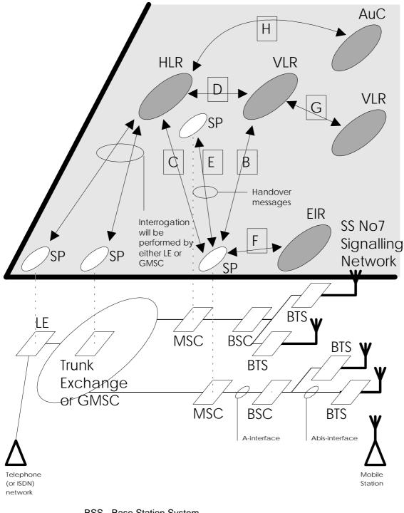
BSS - Base Station System BSC - Base Station Controller BTS - Base Transceiver Station
