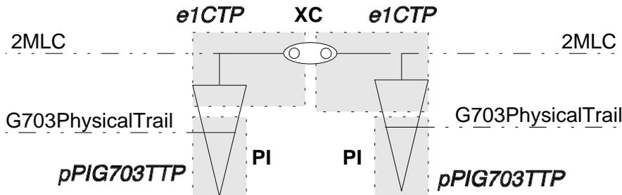
Figure 29: Transfer of an unstructured CCITT Recommendation G.703 [1] / 2 048 kbit/s
