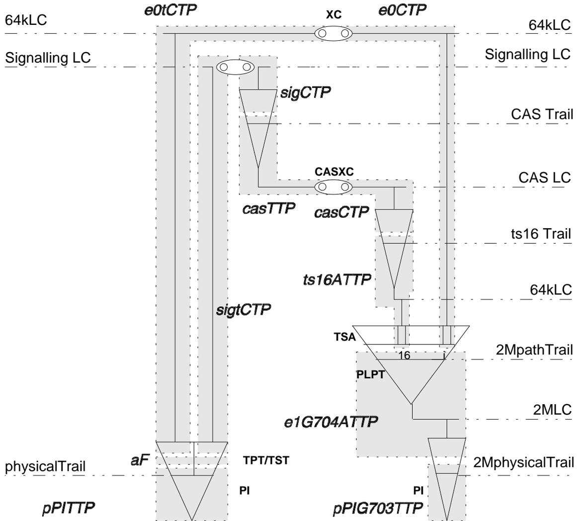
Figure 19: CAS cross-connection between tributary and aggregate
