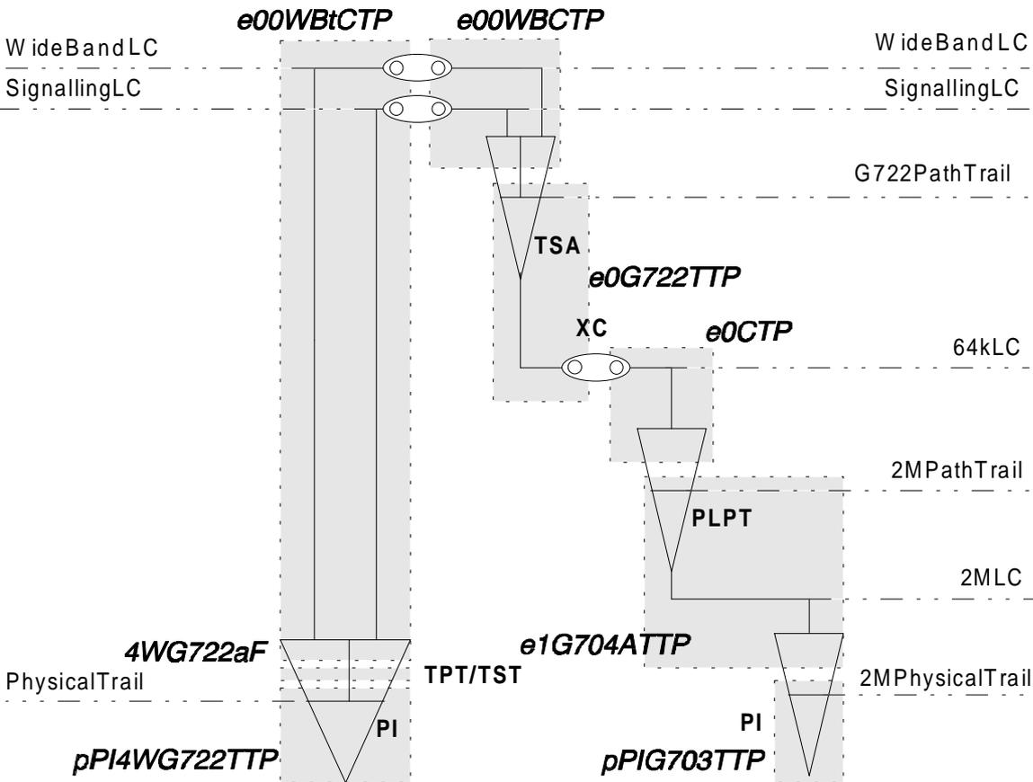
Figure 28: Wide band signal adaptation with signalling
