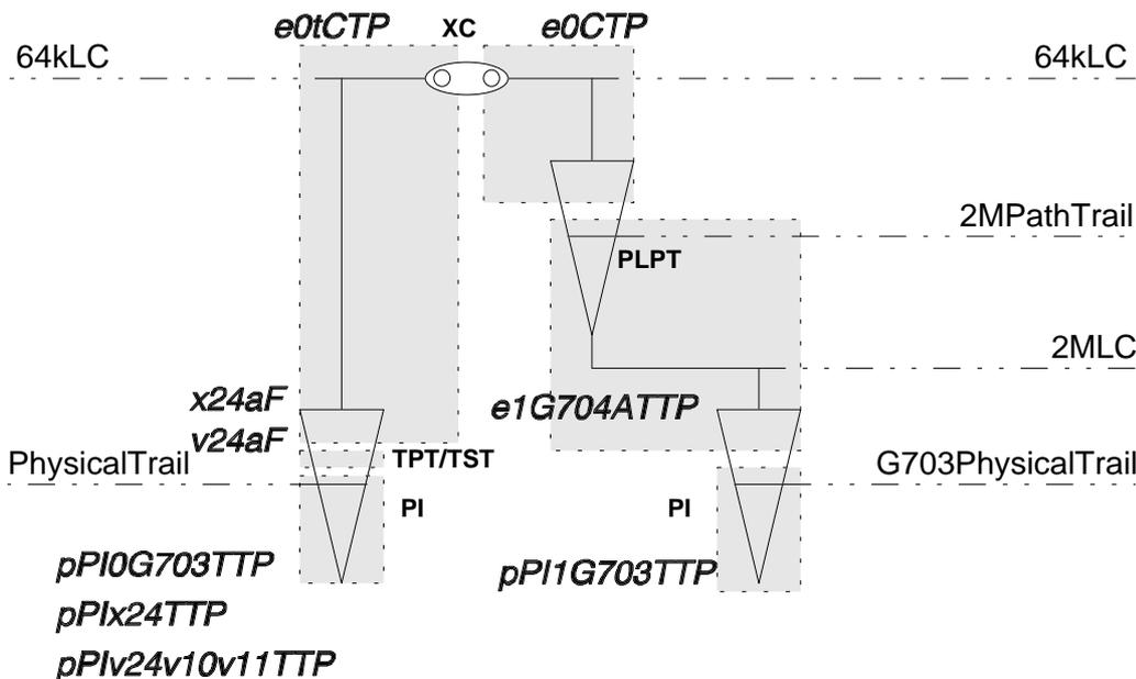
Figure 15: 64 kbit/s cross-connection between tributary and aggregate
