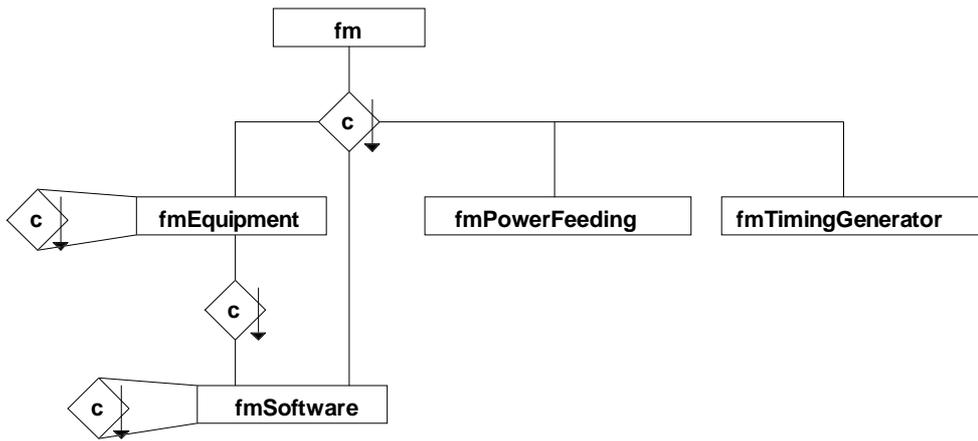
Figure 44: Entity relationship diagram. FM managed element
