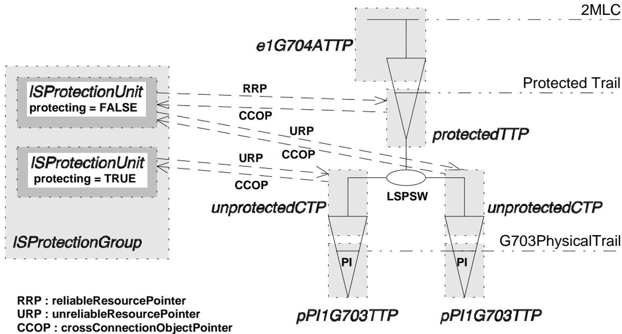
Figure 22: Lower order section protection switch (1+1)
