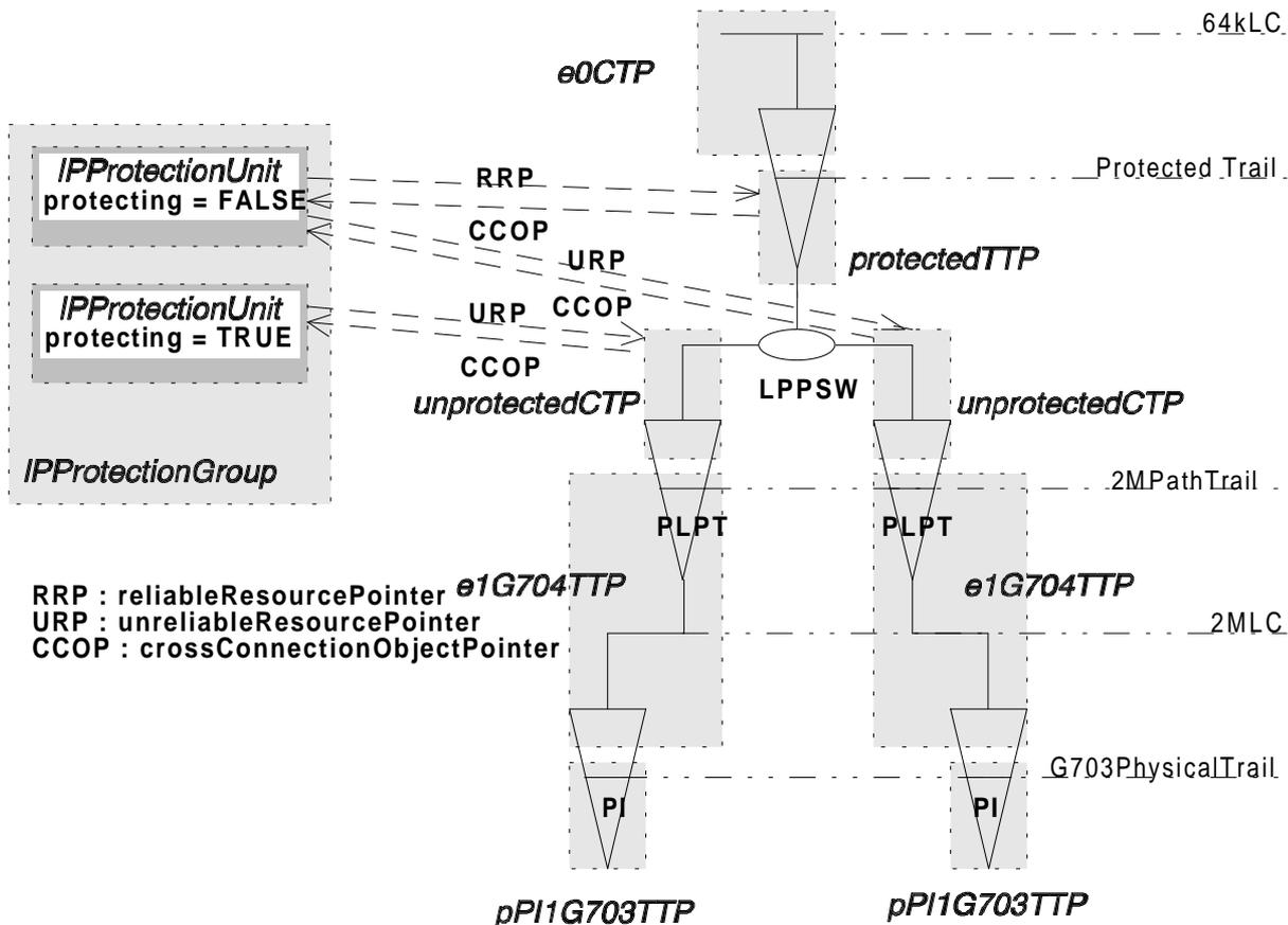
Figure 23: Lower order path protection switch (1+1)
