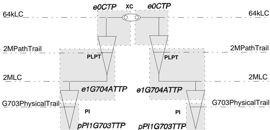
Figure 17: 64 kbit/s cross-connection between ITU-T Recommendation G.704 [2] tributary and aggregate
