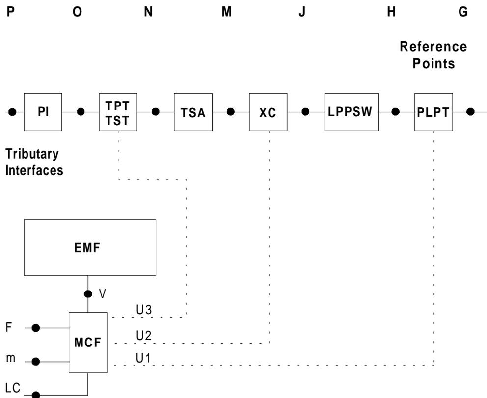
Figure 2: Access to management functions for a FM
