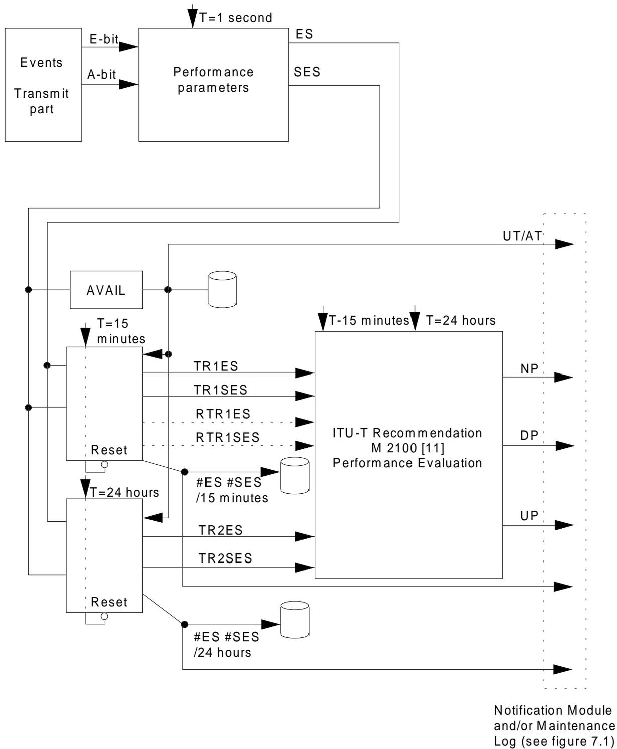
Figure 12: General performance diagram - transmit part
