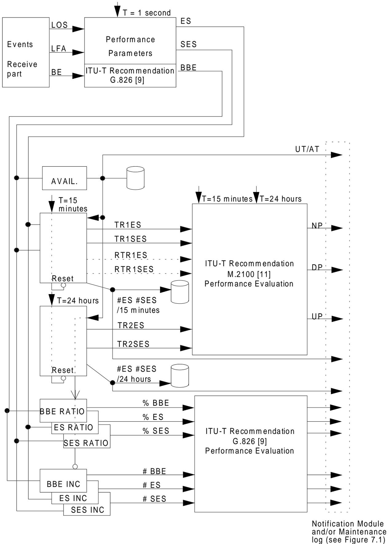
Figure 13: General performance diagram - receive part
