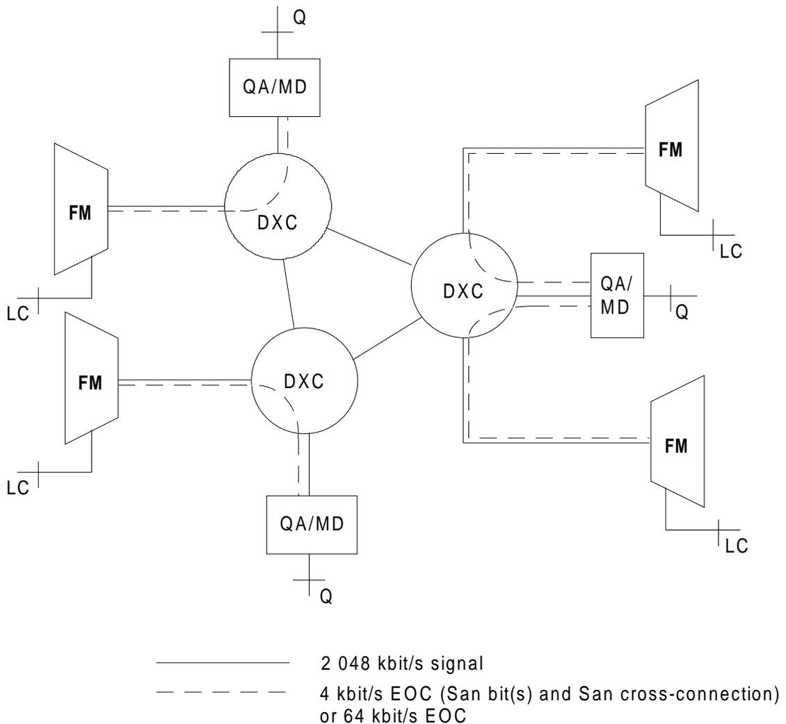
Figure 3: A possible configuration for a FM management network
