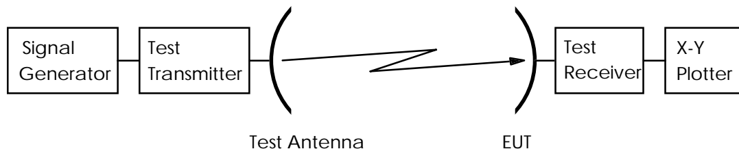
Figure 28: Test arrangement - receive polarisation discrimination
