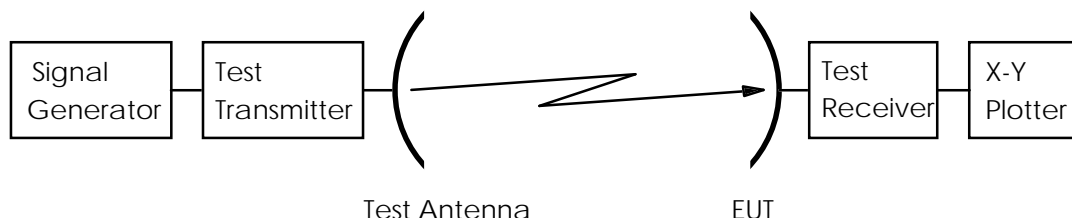
Figure 9: Test arrangement - antenna transmit radiation pattern measurement
