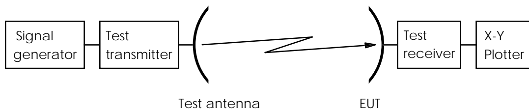
Figure 12: Test arrangement - transmit polarisation discrimination
