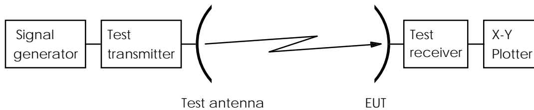
Figure 11: Test arrangement - antenna receive radiation patterns measurement
