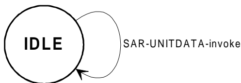
Figure 7: State transition diagram for the SAR Sender
