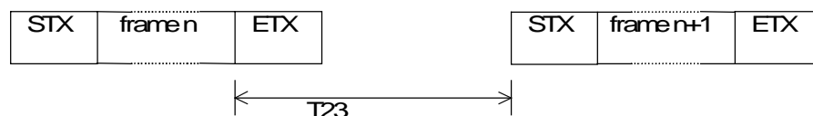
Figure C.3: The time between two consecutive frames
