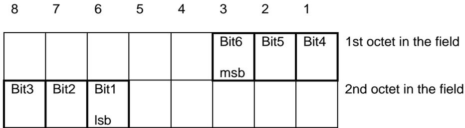
**Figure 90: Field mapping**
