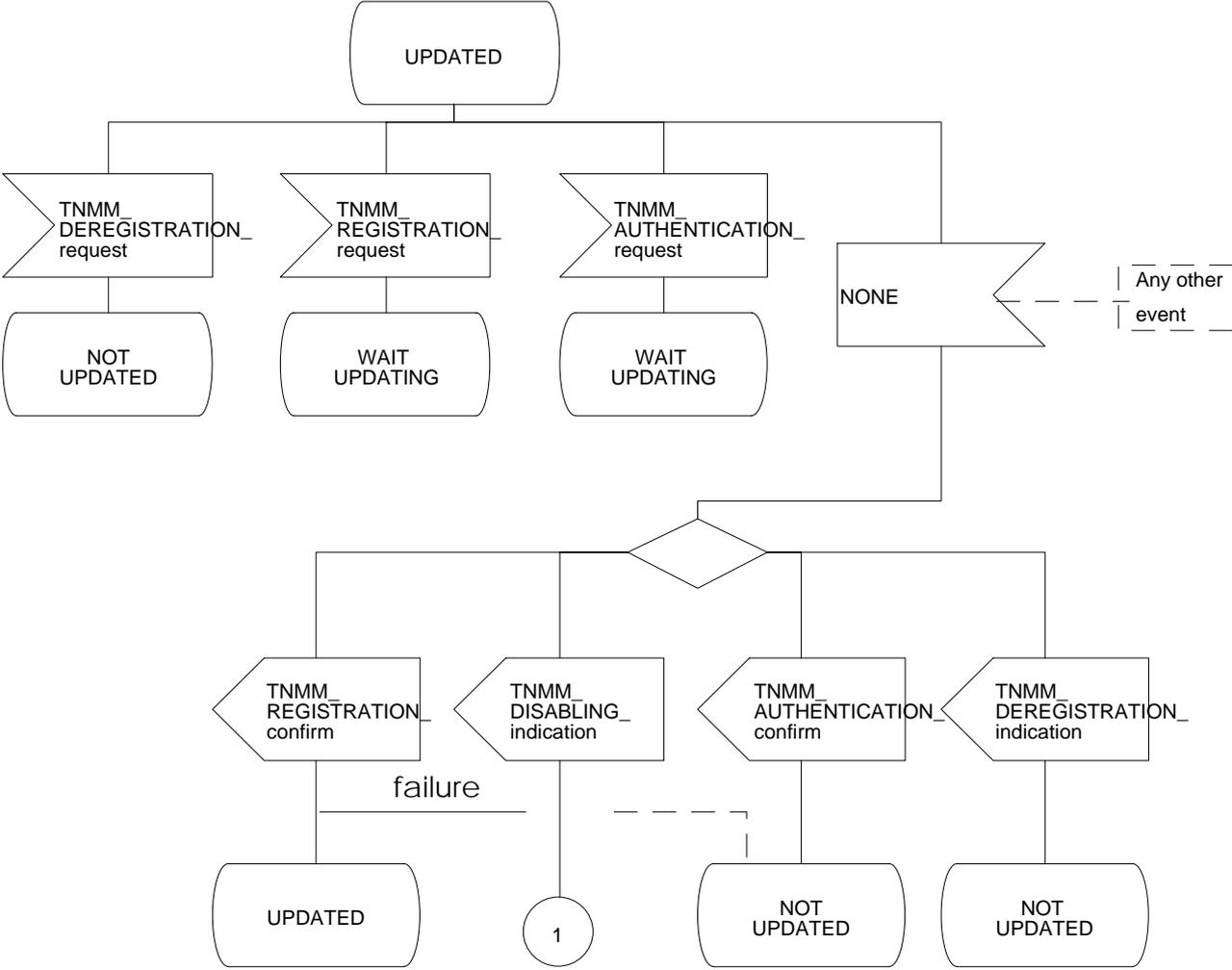
Figure 44: MM service state diagram (sheet 3 of 4)
