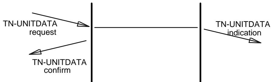
Figure 31: Sequence of primitives for basic data transfer
