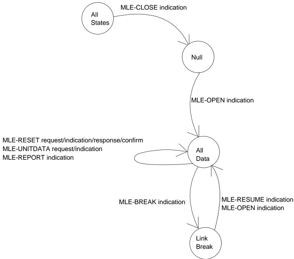
Figure 58: State transition diagram of LCO SAP
