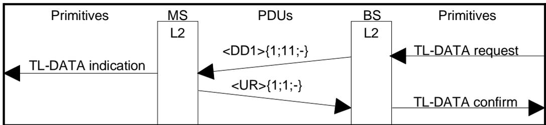
Figure J.6: Acknowledged downlink transfer
