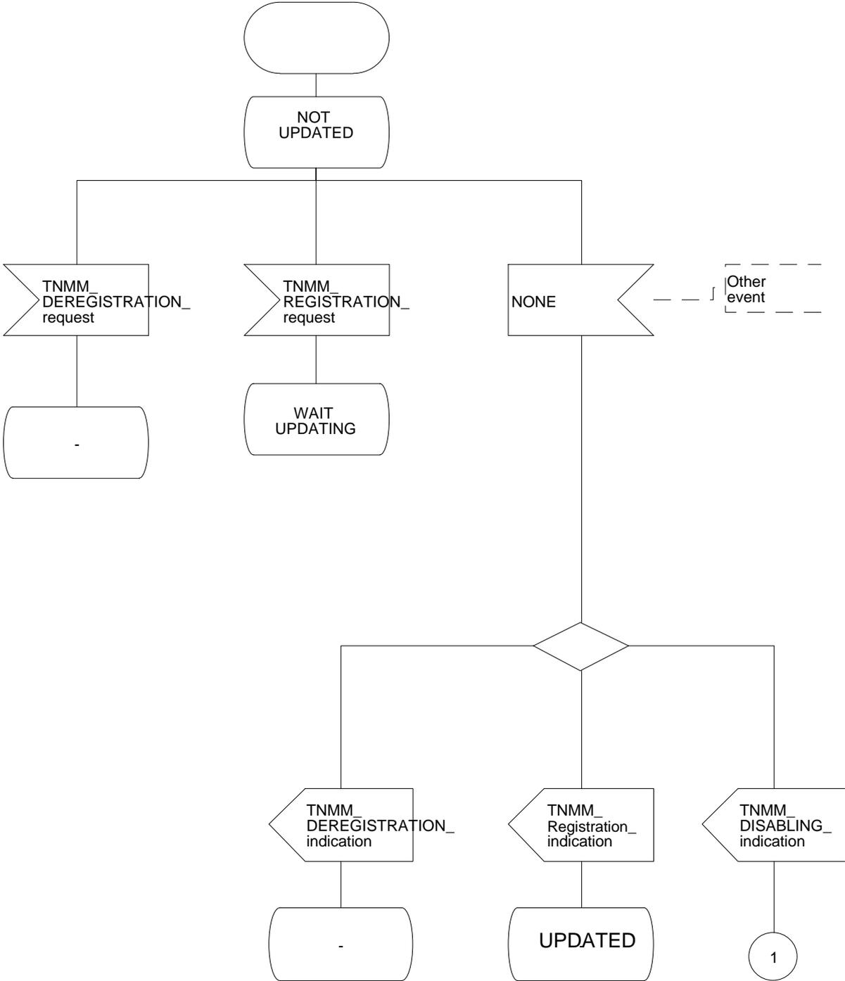
Figure 42: MM service state diagram (sheet 1 of 4)
