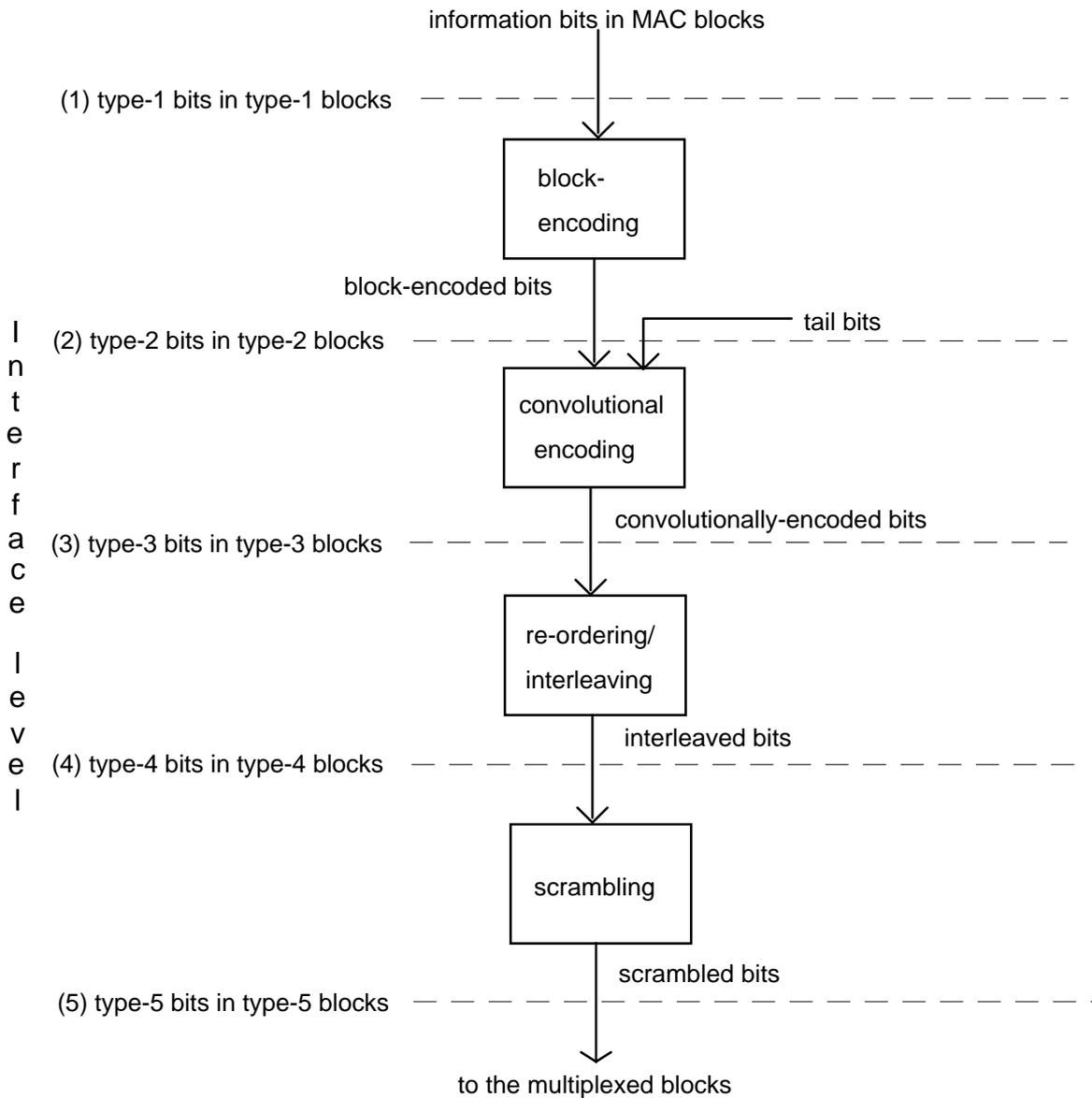
Figure 9: Interfaces in the error control structure
