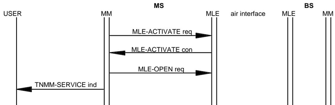
**Figure 47: MM Activation procedure, Registration not supported**
