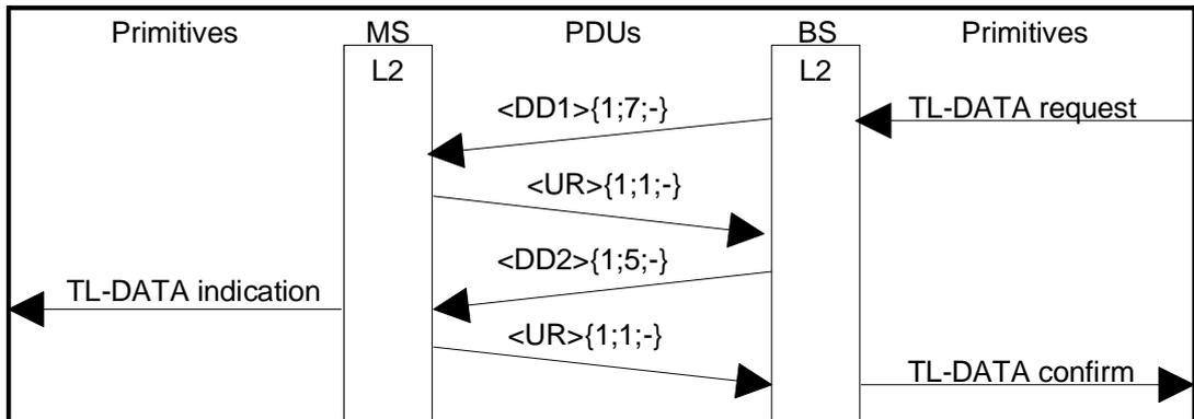
Figure J.7: Acknowledged downlink transfer. Two bursts
