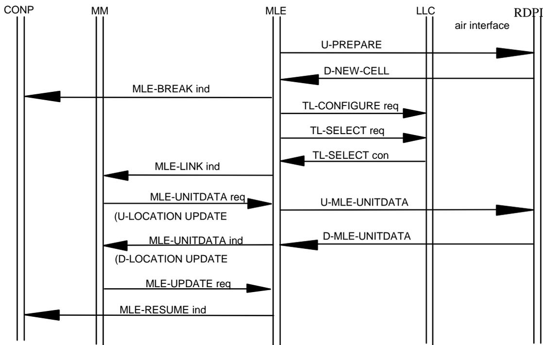
**Figure 67: Announced type 2 cell re-selection procedure**
