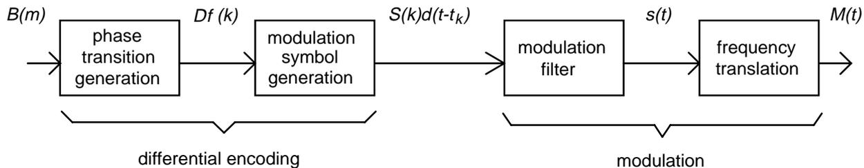
Figure 5: Block diagram of the modulation process
