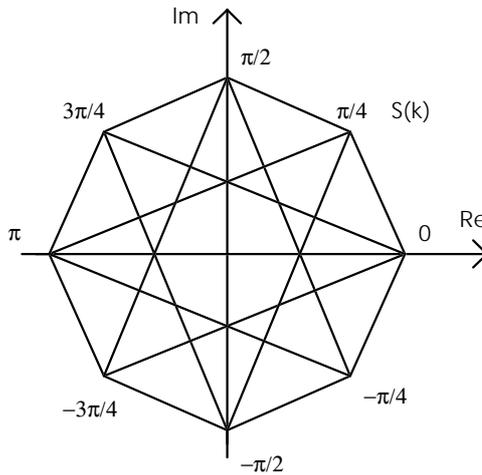
Figure 4: Modulation symbol constellation and possible transitions
