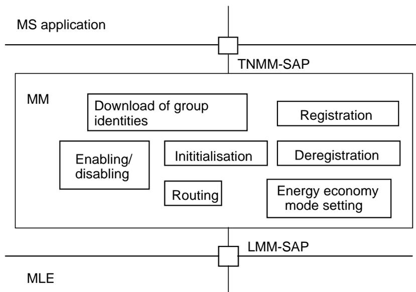
**Figure 46: MM main functions on the MS**
