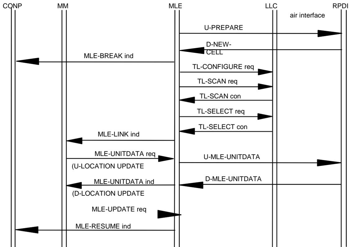
Figure 66: Announced type 3 cell re-selection procedure
