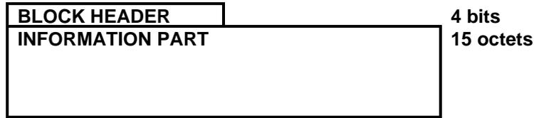
**Figure 71: Structure of the following block**
