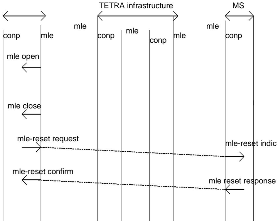
Figure 28: Access to resources and reset protocol sequence
