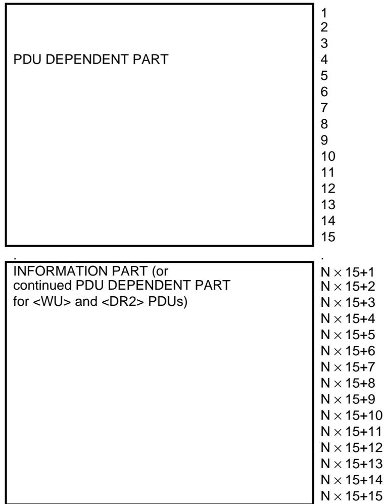
Figure 75: Structure of a variable length PDU, with N the number of following blocks
