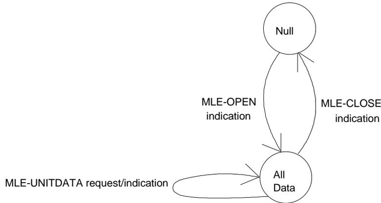
Figure 57: State transition diagram of LSCL SAP
