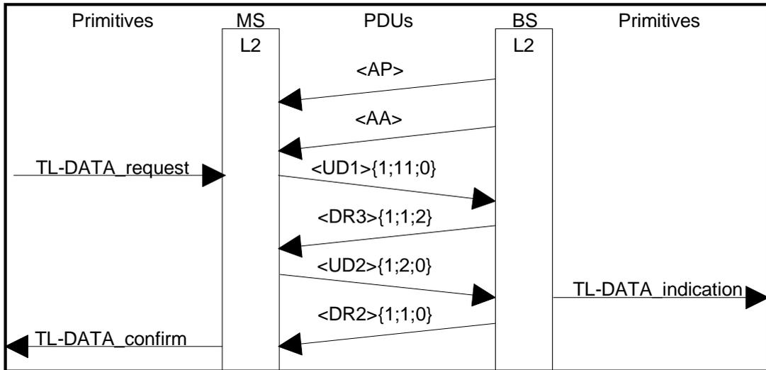
**Figure J.2: Acknowledged uplink data transfer. Busy flag mode. Retransmission of one block**
