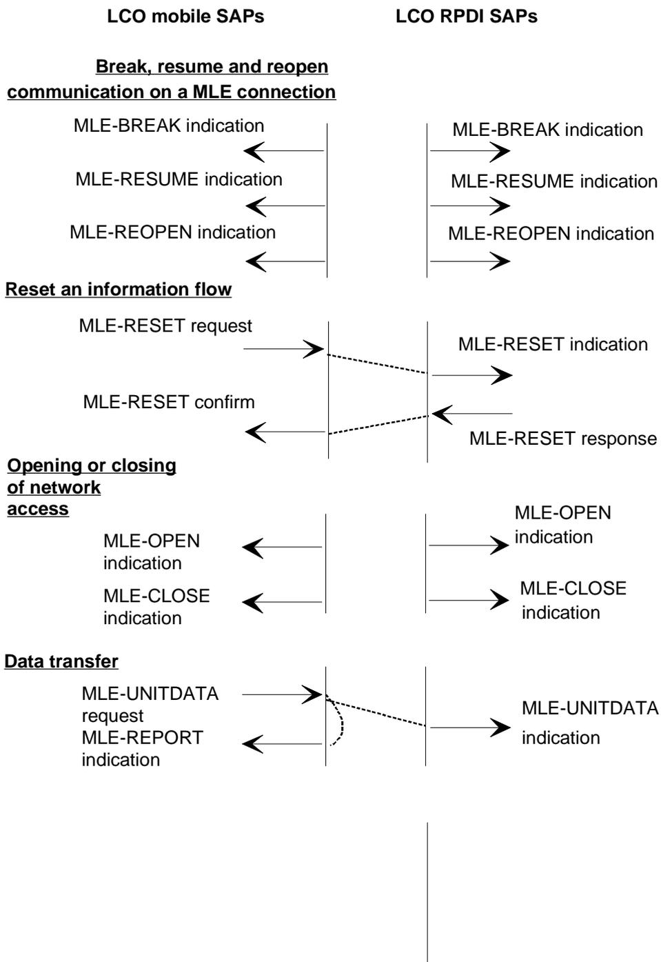
Figure 62: Primitive time sequence at the LCO-SAP
