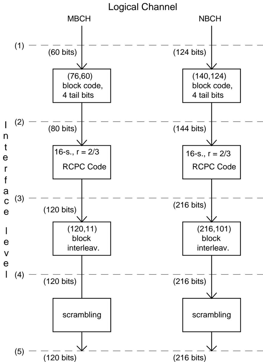
Figure 10: Error control structure for PDO logical channels
