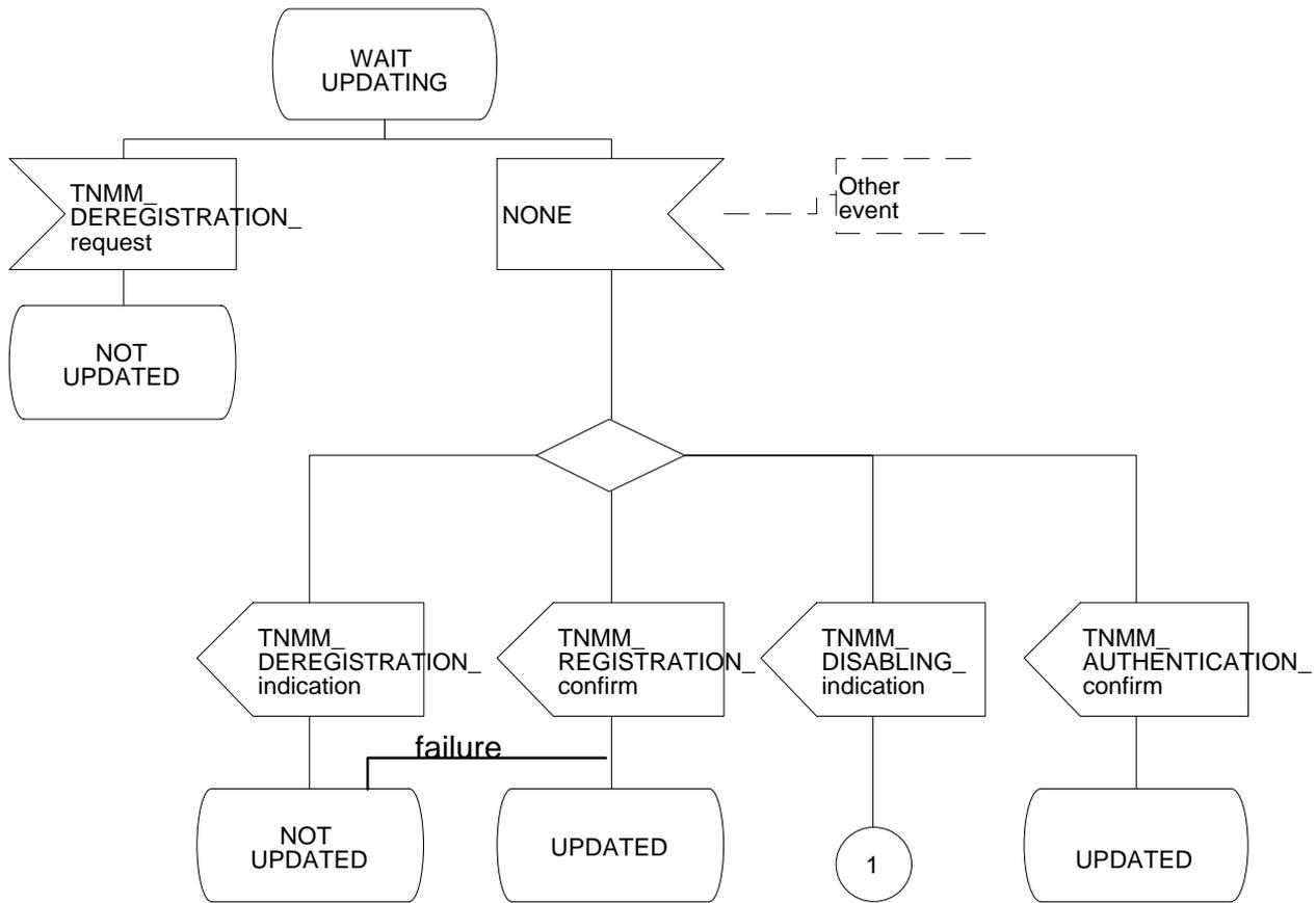
Figure 43: MM service state diagram (sheet 2 of 4)
