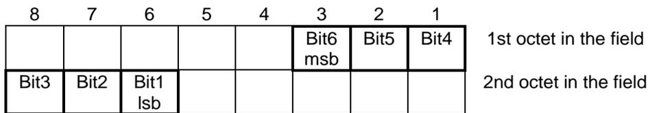
Figure 34: Field mapping
