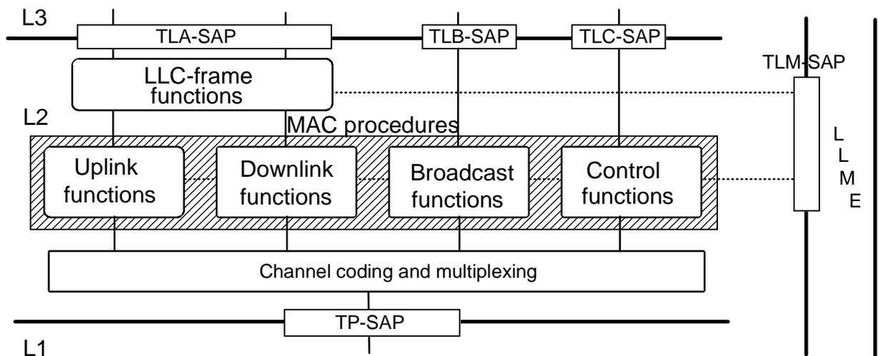
Figure 128: Grouping of layer 2 functions
