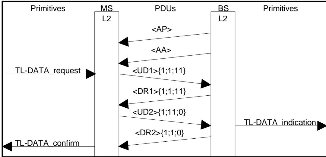
**Figure J.1: Acknowledged uplink data transfer. Slotted Aloha**
