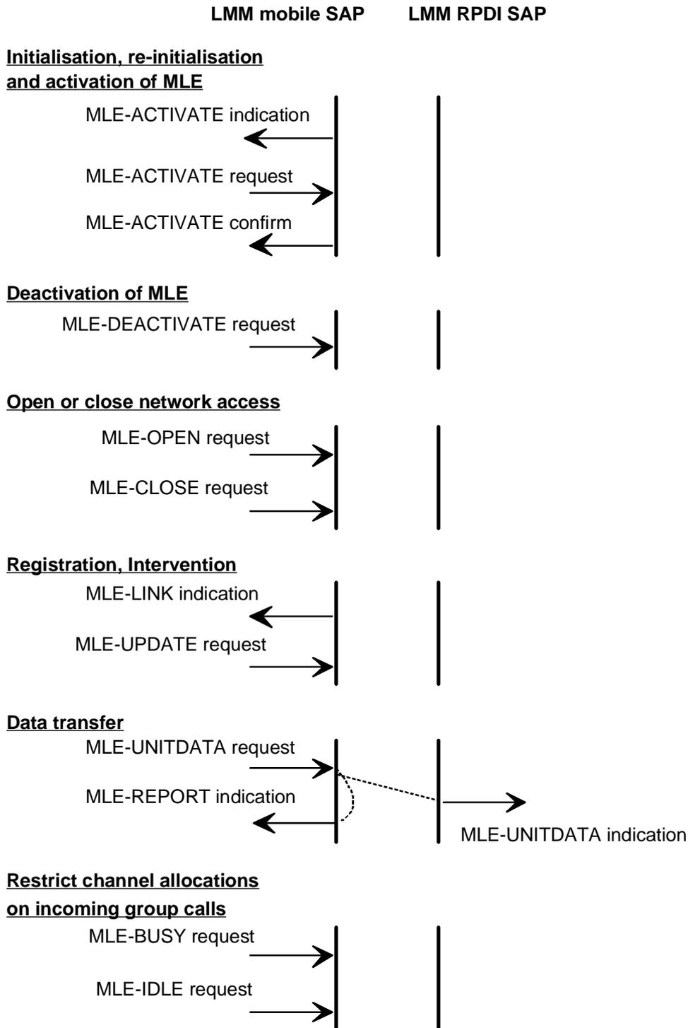
Figure 60: Primitive time sequence at the LMM-SAP
