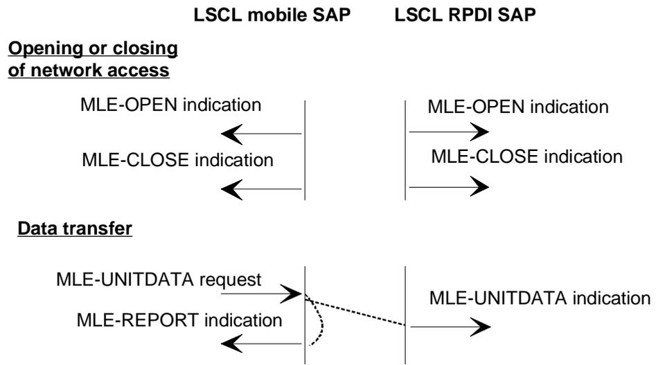
Figure 61: Primitive time sequence at the LSCL-SAP
