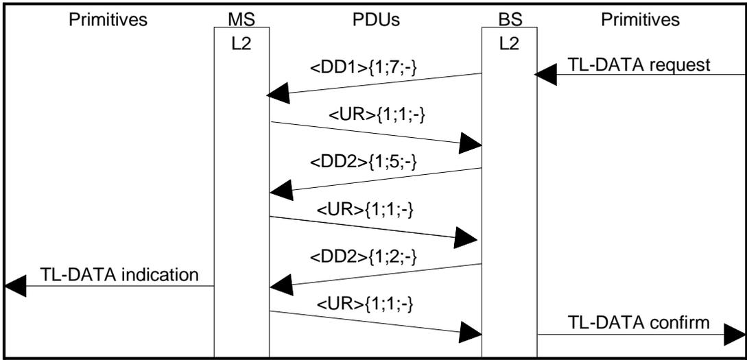
Figure J.8: Acknowledged downlink transfer. Two bursts. Retransmission of one block
