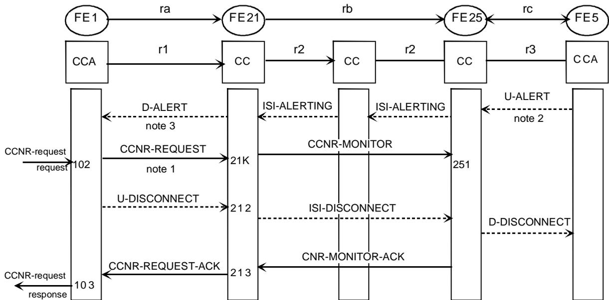
NOTE 1: This example shows invocation of SS-CCNR before releasing the original call. If SS-CCNR is invoked after releasing the original call, CCNR req/ind will occur later than the U\_DISCONNECT and the network will have to keep the information relating to the call just disconnected.
