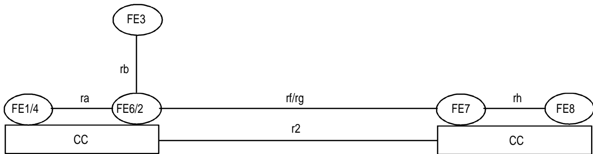
Figure 5: Example relationship between models for ANF-ISIIC and basic call in the case of called user hSwMI being SwMI B, with no migration
