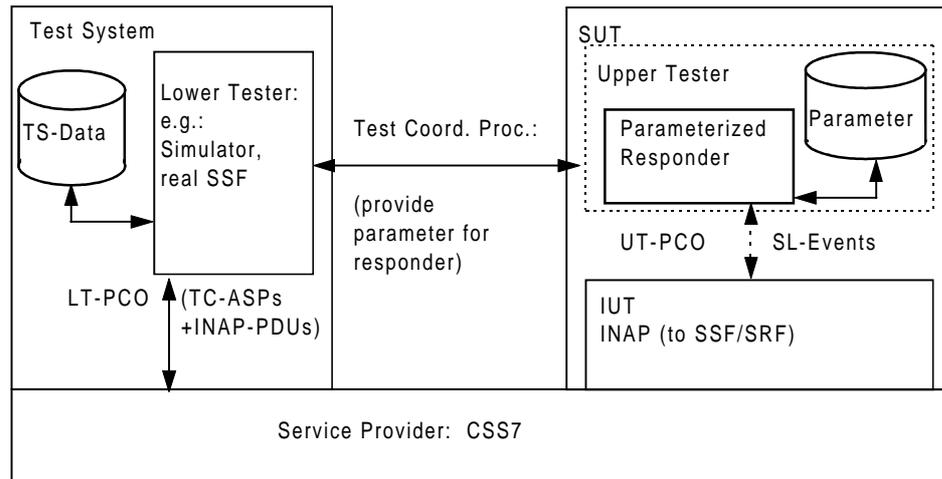
**Figure C.1: Test Configuration of Distributed Test Method**
