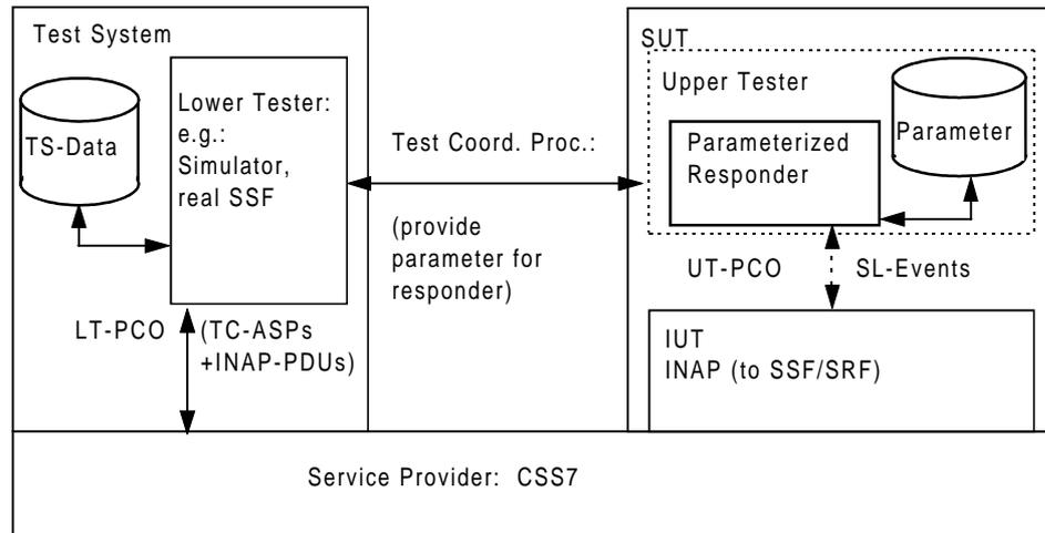
**Figure C.1: Test Configuration of Distributed Test Method**
