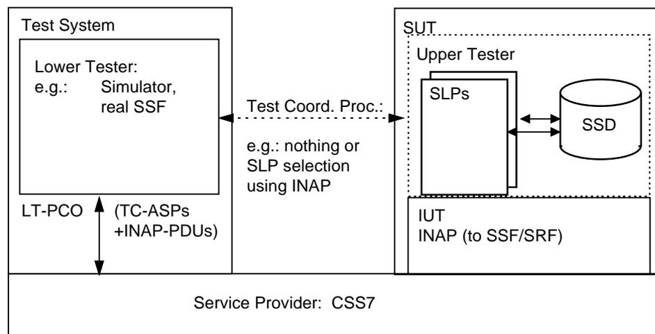
Figure C.2: Test Configuration of Remote Test Method
