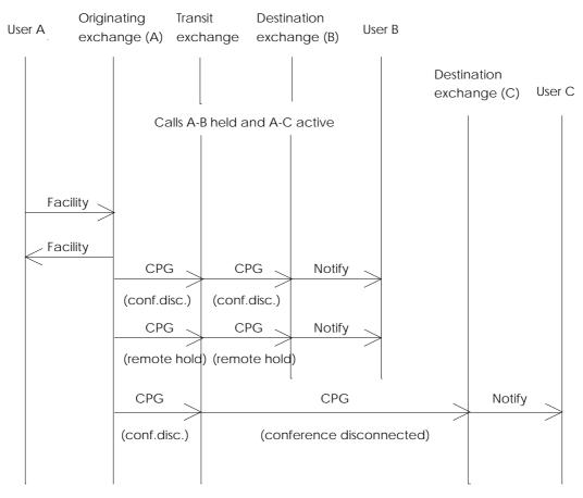
NOTE: The signalling flow for creating a private communication with user B is different, and follows that given in ETS 300 188-1 [5].
