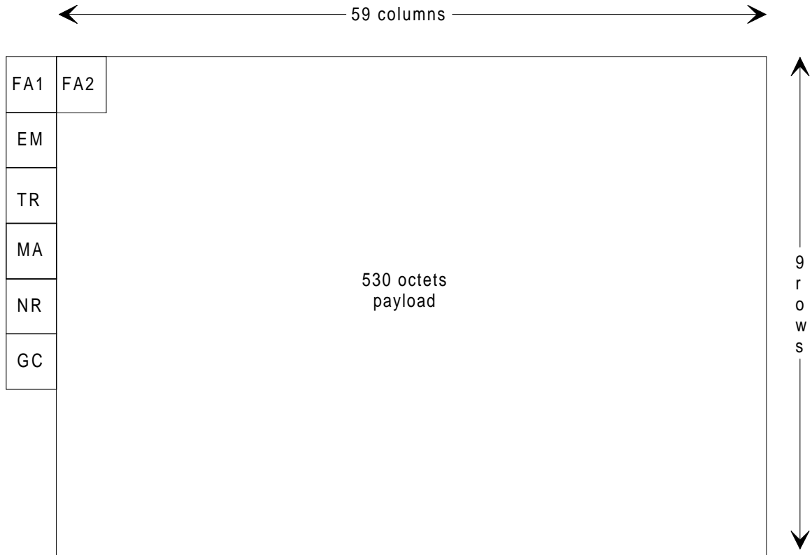
Figure 2: Frame structure at 34 368 kbit/s
