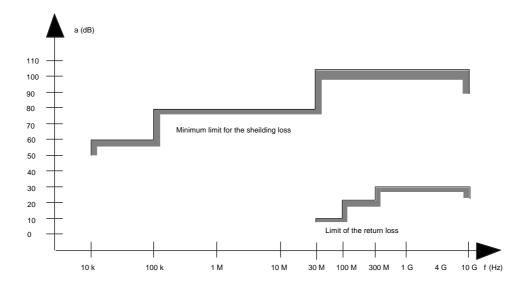
Figure A.2: Specification for shielding and reflections
