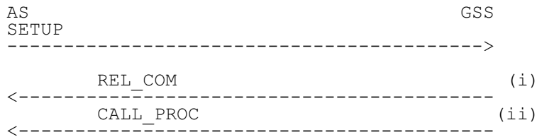
Figure 52: Aircraft originated call initiation and possible subsequent responses
