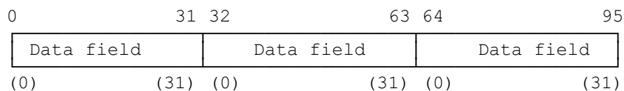
Figure 15: G3 Slot twelve octet data format
