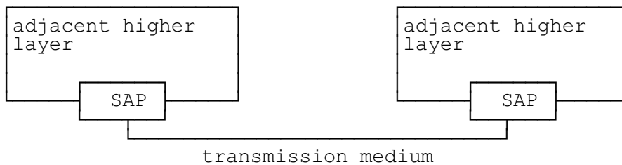
Figure 7: Service Access Point
