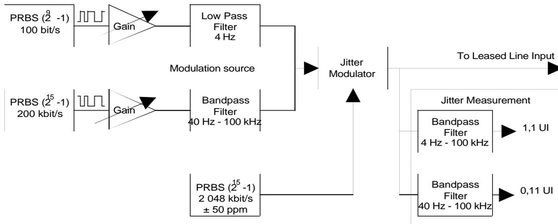
Figure A.4: Input jitter generation
