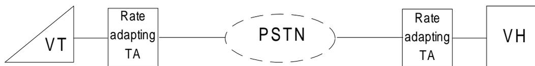
Figure A.2: Access of PSTN/PSPDN systems via rate adapting terminal adaptors
