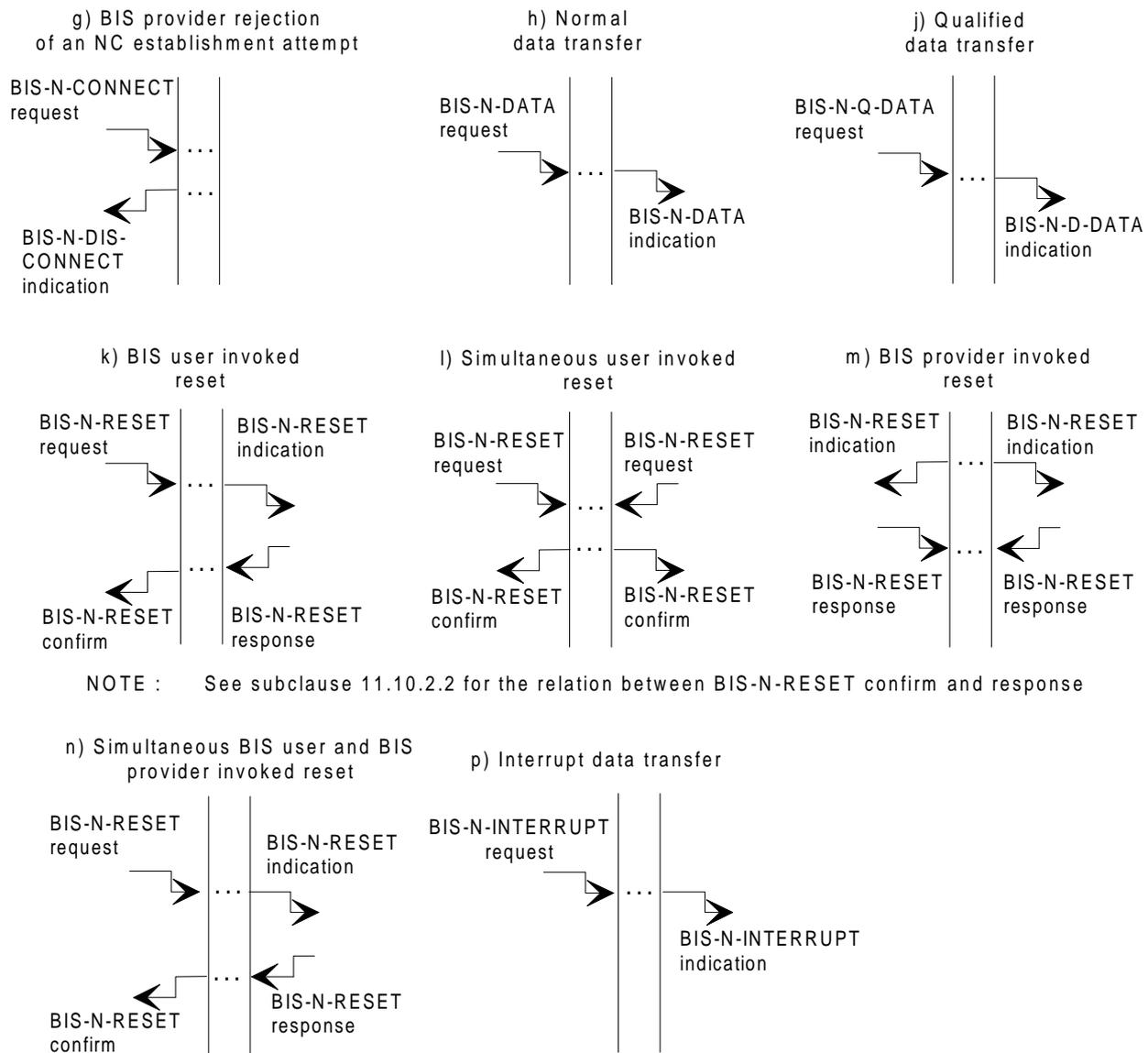
Figure 15: Summary of BIS service primitive time sequence diagrams (concluded)
