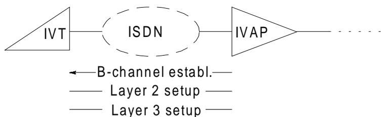
**Figure A.15: Host to terminal connection establishment**
