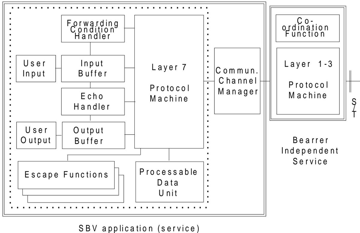
NOTE: For every communication channel, one separate independent instance of each of the functional entities inside the dotted rectangle exists.
