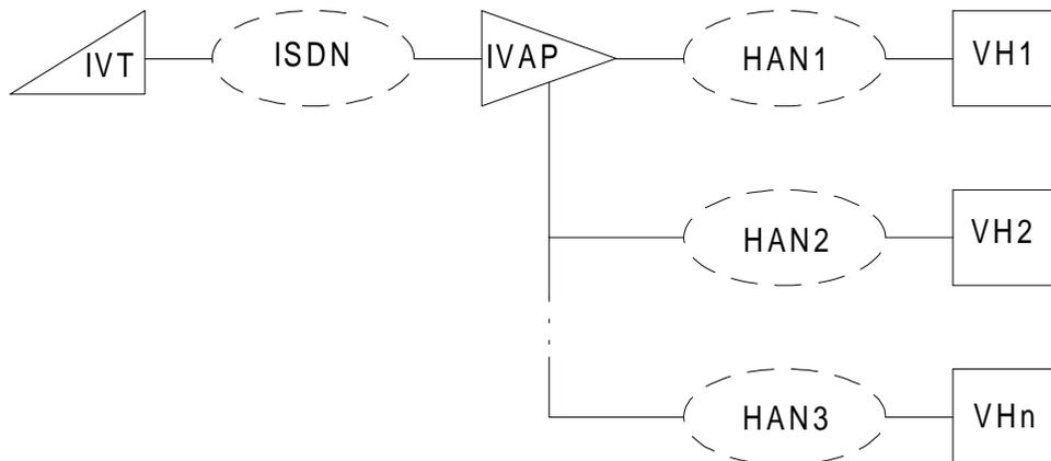
**Figure A.11: Distributed Videotex Host configuration**
