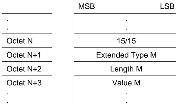
**Figure 8: Extended coding structure**
