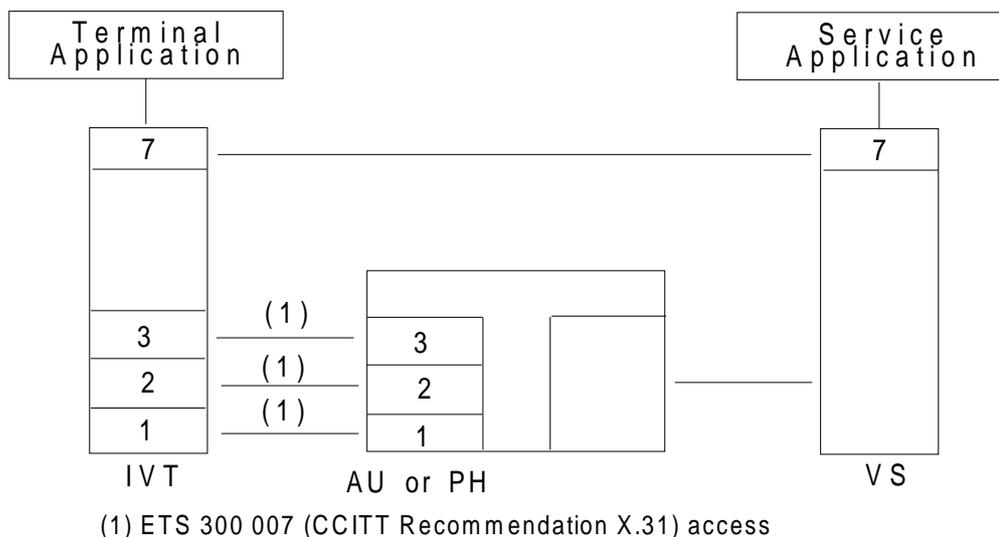
Figure A.6: Protocol stack for IVT-AU/PH-VS connection
