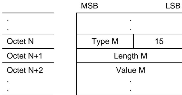
**Figure 7: Basic coding structure with length extension mechanism**
