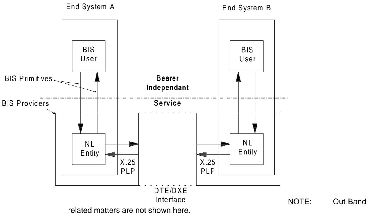
**Figure 14: Operation of the BIS**
