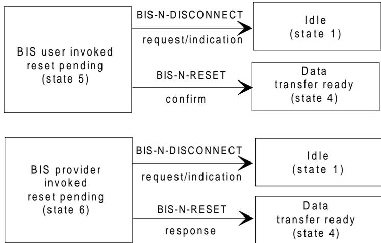
Figure 16: State transition diagram (concluded)
