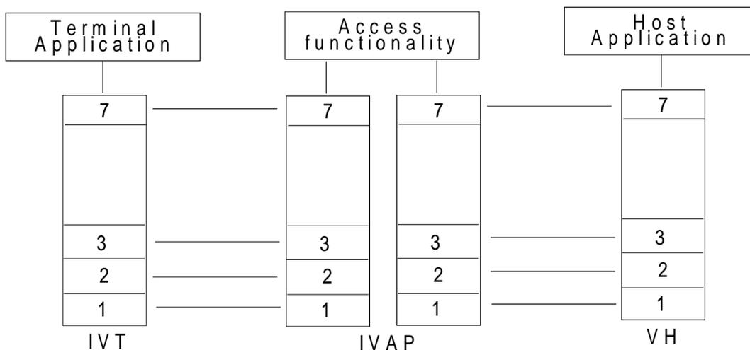
Figure A.8: Protocol stack for IVT-IVAP-VH connection
