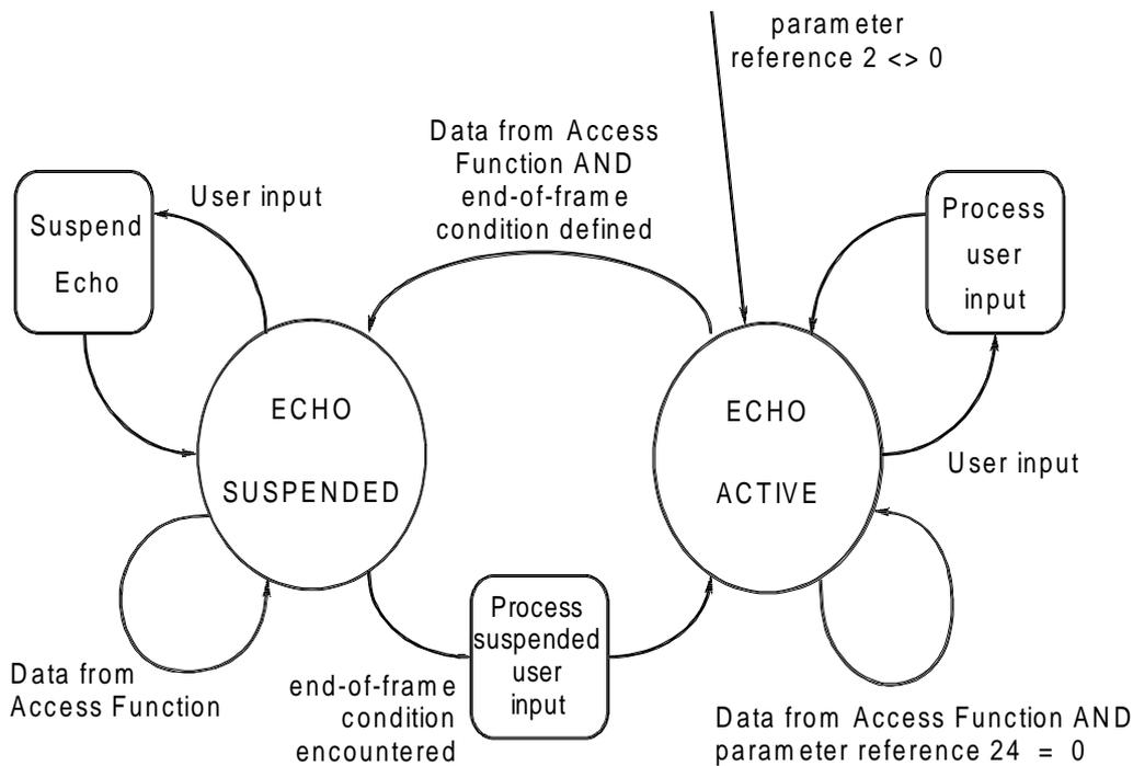
NOTE: An end-of-frame condition is defined if either CCITT Recommendation X.3 [3] extended parameter reference 24 is not implemented or if parameter reference 24 has been set to a non-zero value.
